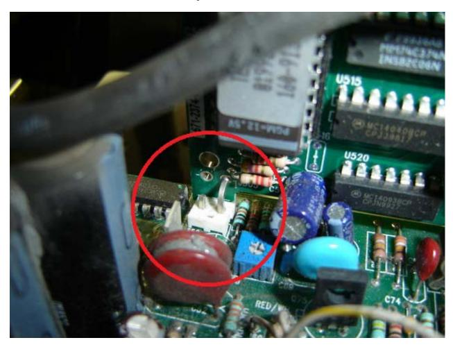
3: Add two new ground terminals inside the CRT driver compartment.
